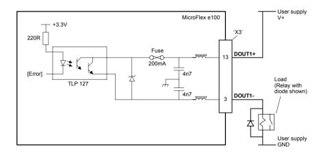
Figure 32 - DOUT1 output circuit
